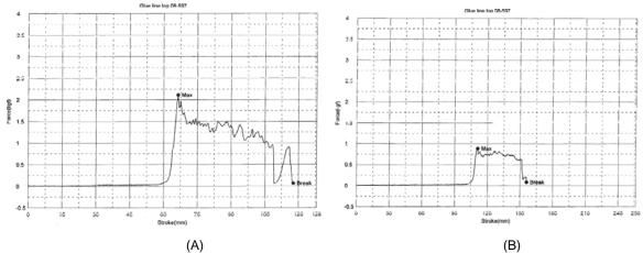
Figure 3. Glue peel strength of (A) new element and (B) element operated on produced water feed for six months at pH = 10.7 and temperature = 35 C.
